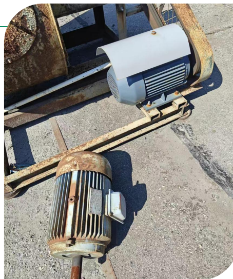
▲ High-energy-consuming motor replacement (before and after comparison)
